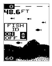
The Fish ID feature can't be used when the unit is in the manual mode. If you turn the automatic feature off, the Fish ID feature will automatically be turned off, also.
